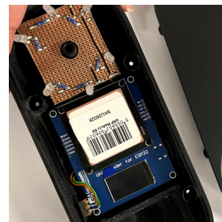
Lay UHF RFID Reader and push PCB into snap fits
